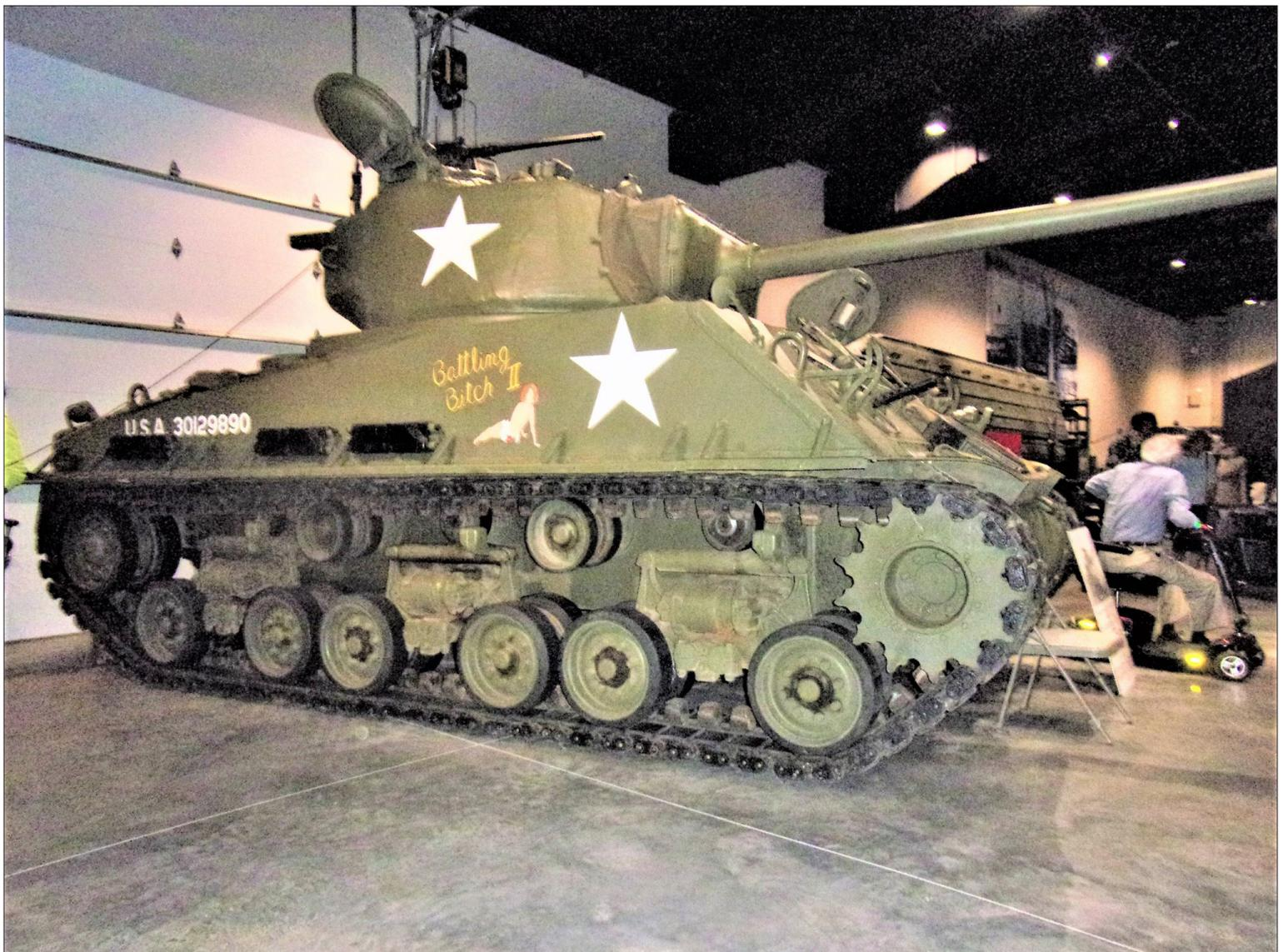
The 1945 M4A2 Sherman tank Easy model with 76 mm main gun. Twin 6 cylinder General Motors Diesel engines, built by Fisher Body. Requires five crew members to operate. Equipped with: 1-50 caliber machine gun mount on turret. 1-30 caliber machine gun M1919 in turret. One 30 caliber machine gun M1919 in Beaumont. Five-45 Waksman M3. Combat loaded weight 73,400 pounds, maximum speed 30 mph. Owned by the Buck family, motor pool at Gettysburg, Pennsylvania.--Bill Wurzell photos
