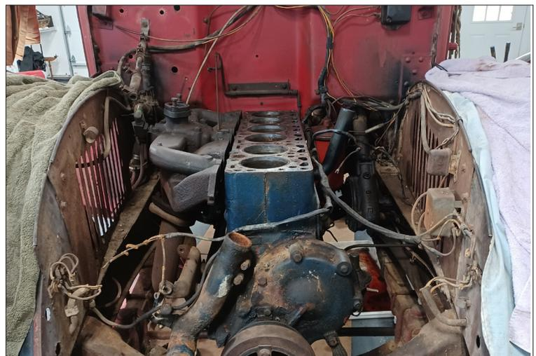
Head and gasket removed from engine block
