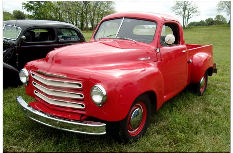
This is one of the nicest examples of a 1949 Studebaker pickup truck I've ever seen. It's a six cylinder flat head, with three-on-the-column, minimum gauges, and dog dish hubcaps.--Bill Wurzell
