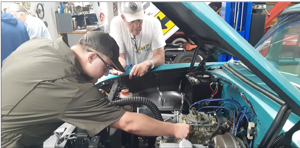
Michael adjusts the fuel mix on the carburetor while Gary Wilmer looks on.
