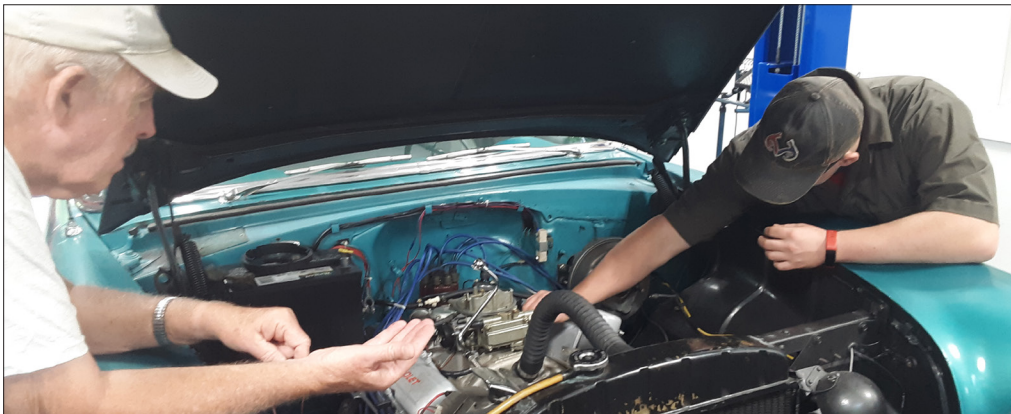
Gary Wilmer instructs Michael how to smooth the idle on the engine so it is at the ideal RPM.
