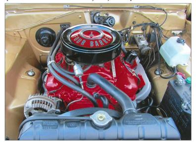
The Barracuda's mighty 340 cubic inch V8, naturally aspirated four barrel carburation. Engine bay is perfection.
