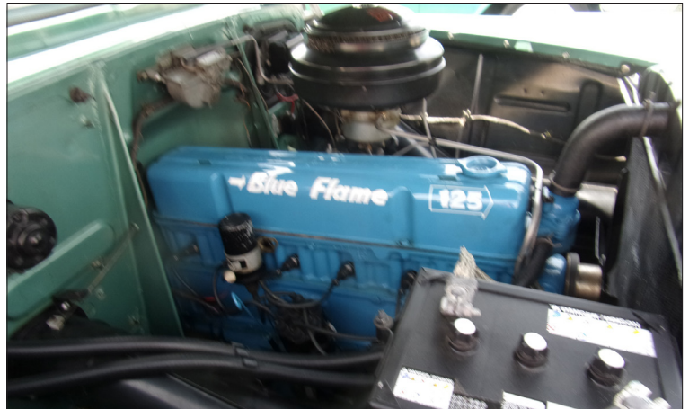
Over the years, Chevrolet constantly made improvements to this OHV six cylinder engine, and it kept Chevy 'in the game' for decades.
