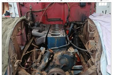
Head and gasket removed from engine block
