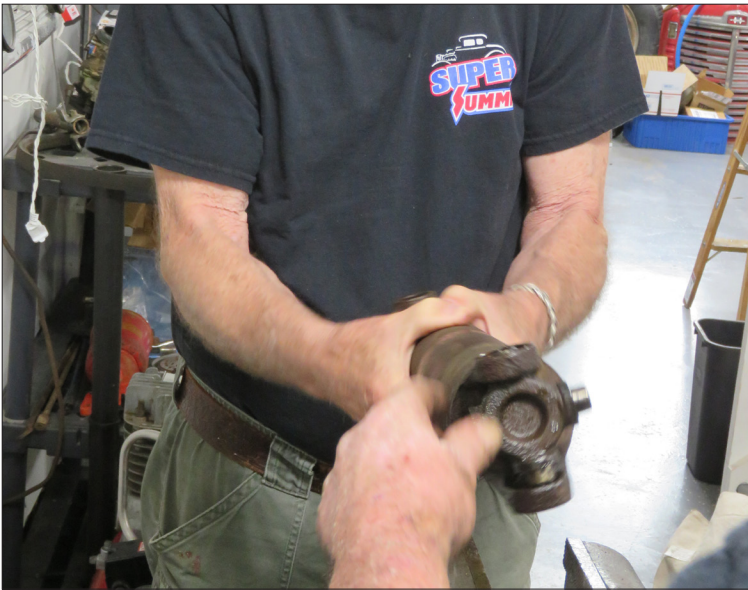
Figure 7: Removing released journal cross. Note trunnion missing its cap.
