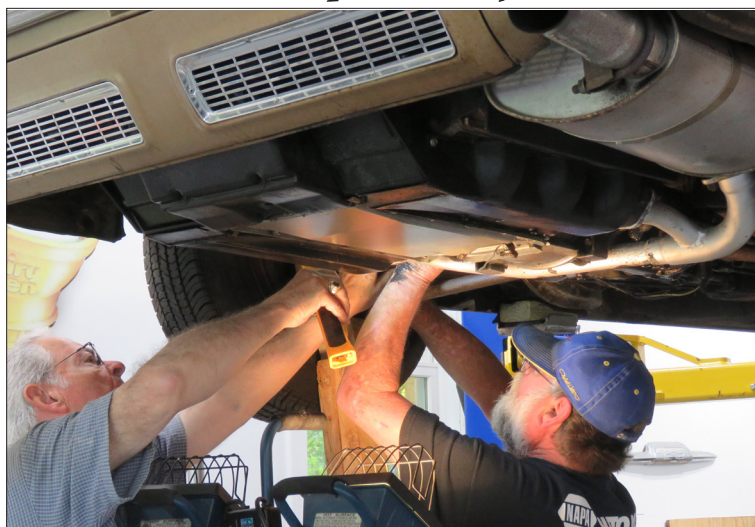
Figure 2: Doug and Mike remove half shaft.
