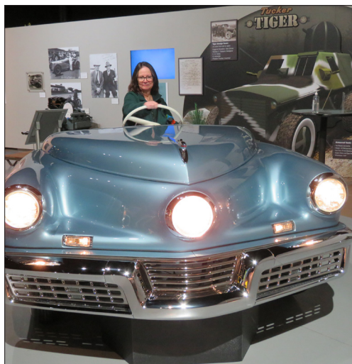
Barb Diehl tries out a Tucker display that features how the center headlight swivels to more effectively 'light up the road.'
